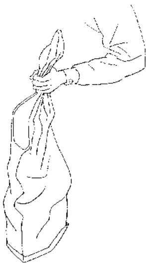
Figure 12A: Sandbag filled 1/4 to 1/3 full
